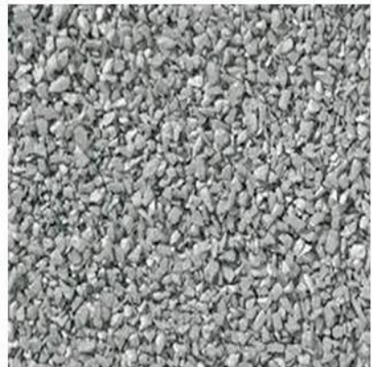
P10 - LOOSE GRAVEL - COLOR-GRAY - FINISH-ROUGH - 10-20MM DIA X50MM THK.
