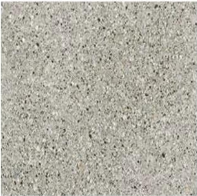
P02 - GRANITE PAVING - COLOR-LIGHT BEIGE - FINISH-FLAMMED - 1200X1200X30MM THK..
